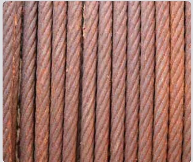
Protecting the rope from the often severely corrosive conditions encountered in marine and other environments is another key consideration. Although ropes may appear in good condition, corrosion of the core may go unnoticed, creating a potentially dangerous situation.
